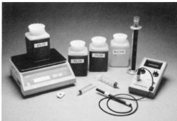
FIGURE D.2.1.2 Equipment Needed for Conductivity Method of Proportioning Measurement.
